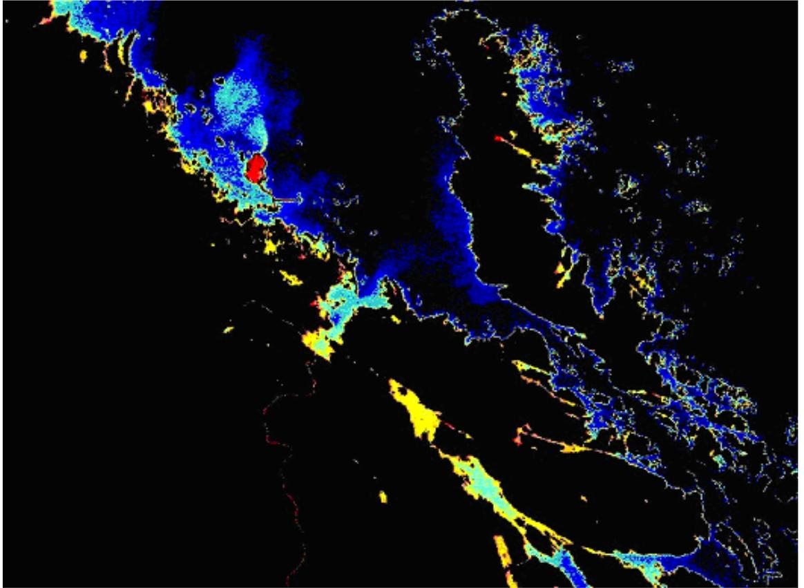
*figure 8. Temperature variation in shallow coastal waters 2003-04-26, close up of Forsmark, Uppsala county. Thermal variation is described from warm (red) to cold (blue). See text for description of classification. Note the cooling water outlet from the Biotest basin at the Forsmark nuclear plant (top left).*
