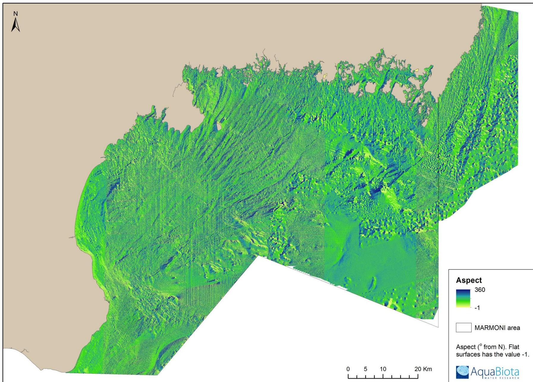
Figure 94. Aspect shown in degrees from the north, based on the interpolated depth grid.
