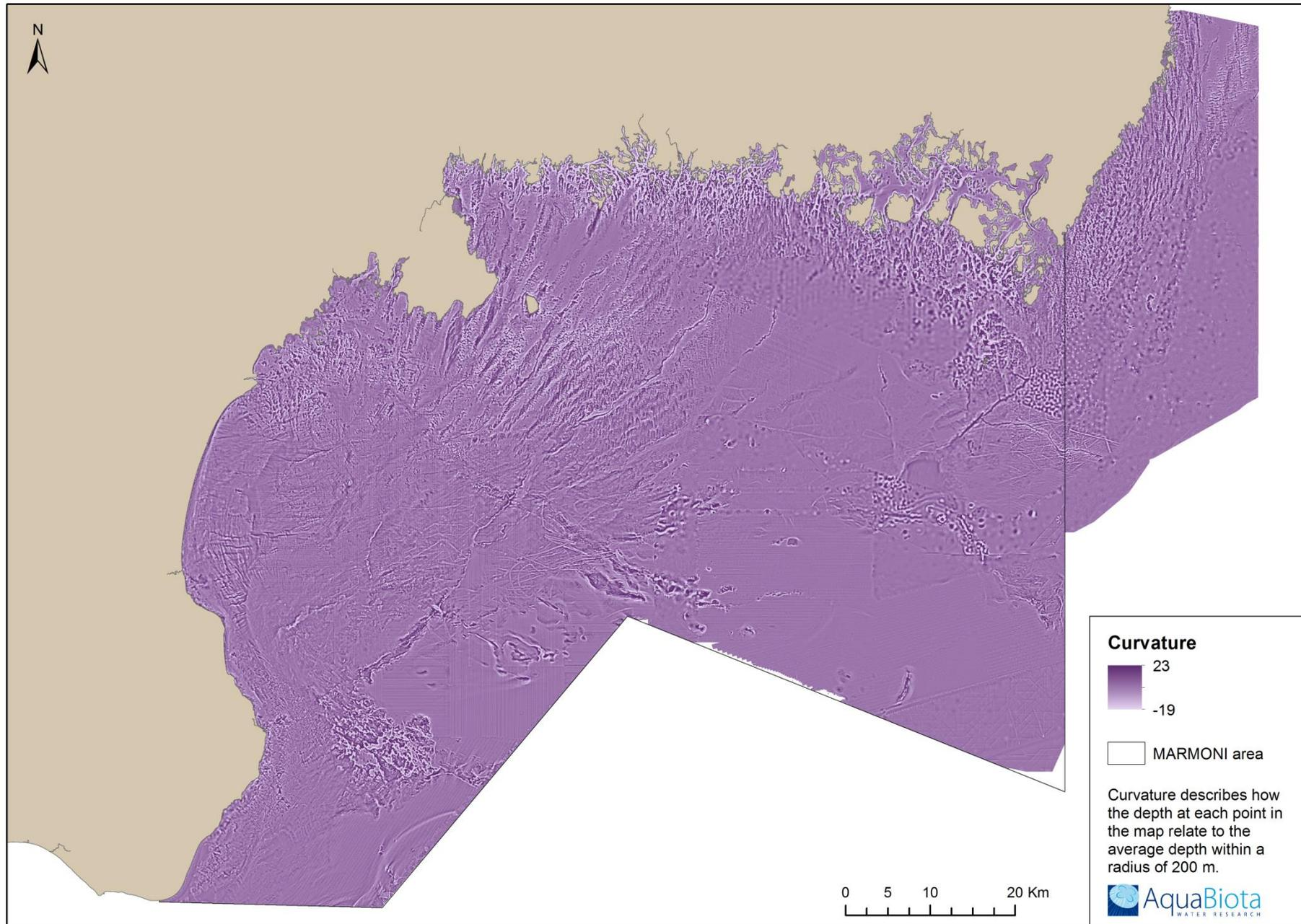
Figure 95. Curvature based on the interpolated depth grid. Negative values illustrate sinks and positive values illustrate hills.
