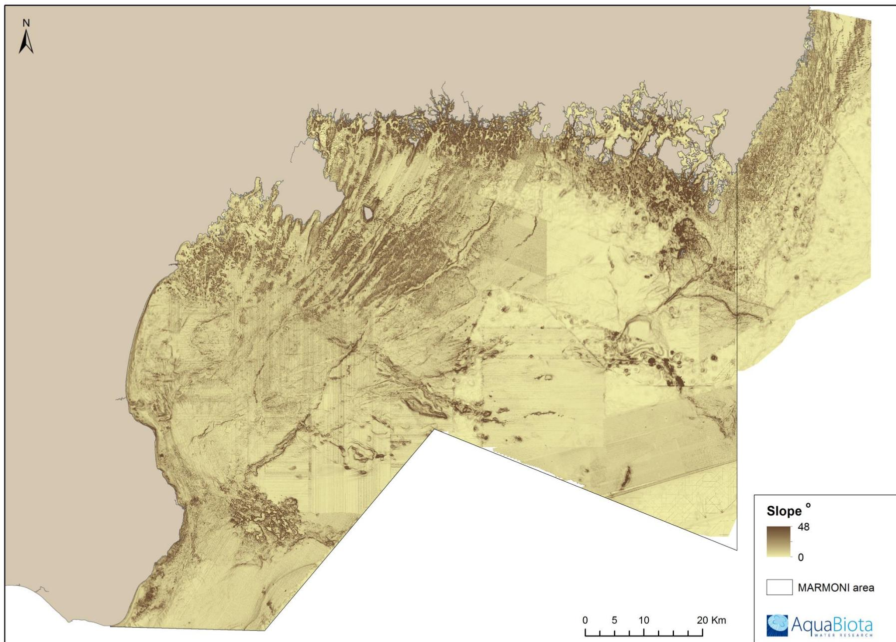
Figure 93. Slope based on the interpolated depth grid. Zero degrees denotes a horizontal surface and 90 degrees a vertical surface.
