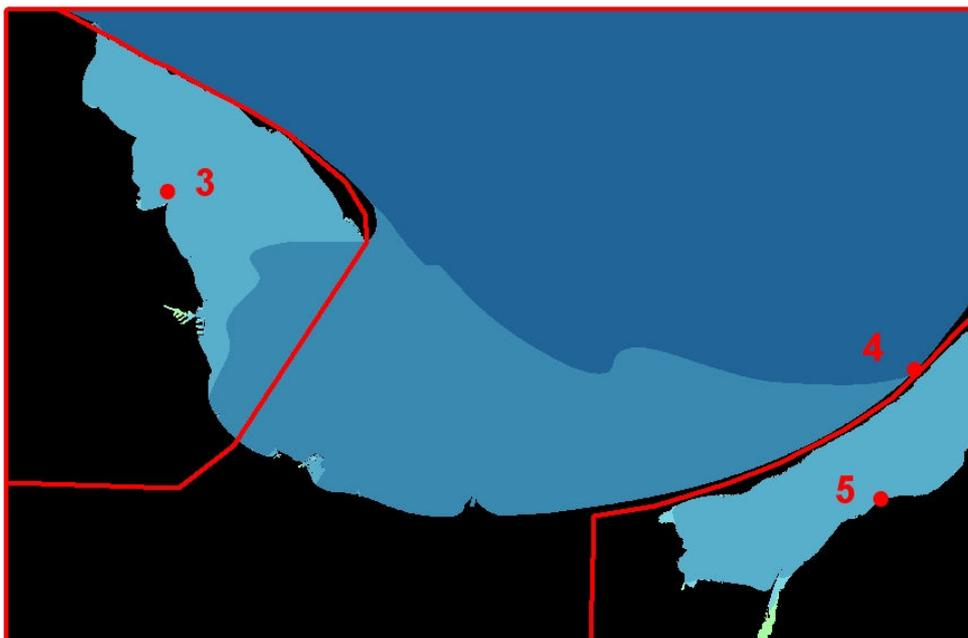
**Figure 5.** The resulting wave exposure of grid 5 is the merged outcome from three separate runs in which different wind stations (V3-V5) were used.
